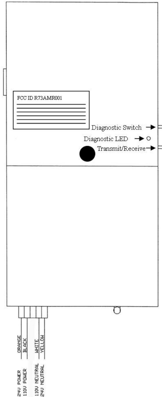
**The V-AW12A and V-AW16A wireless clocks can be powered by 2 "D" cell batteries, 24 volts AC, 110 volts AC, or 220 volts AC.**
