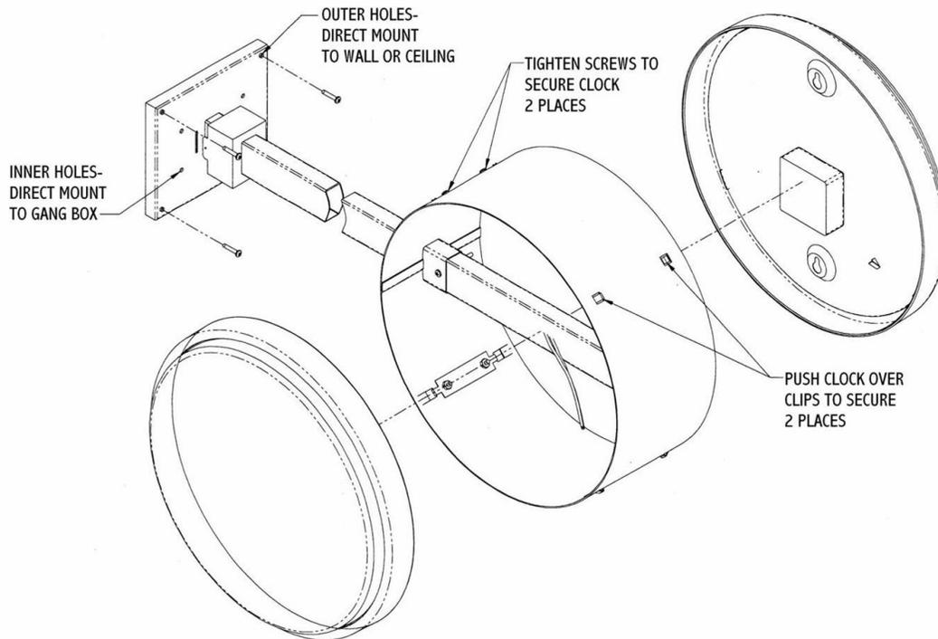
1. Screw the mounting bracket to the double gang box using four (4) inner holes on mounting bracket, or mount the mounting bracket directly to the wall or ceiling using the four (4) outer holes.
