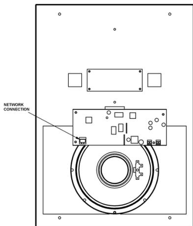
Figure 2. Ethernet Connection
