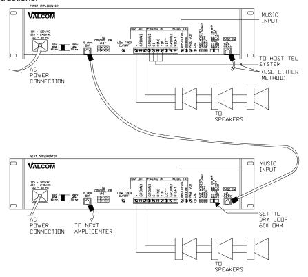
Figure 13. Series Amplicenter Without Controller
