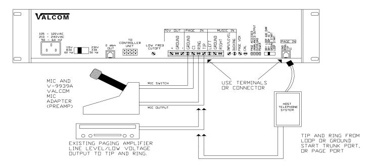
Figure 6. Host Telephone System Connection
