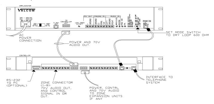
Figure 12. AmpliCenter Interface with PagePac Plus Controller (V-5323100)
