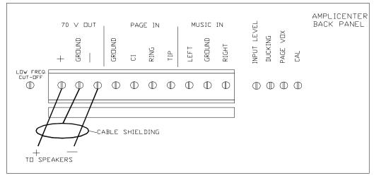
Figure 4. Speaker Connection on AmpliCenter
