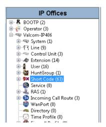
6. Click the New icon in the upper right corner of the Details pane to create a new Short Code. In the Details pane, enter a code that will match the dial code used in your system. For our example, the Valcom VIP-201 will be configured with phone numbers 5801 – 5808, so the Code will be entered as "580X;". Select "Dial" for the Feature. The Telephone Number to send will be 580N" 192.168.96.237", and the Line Group ID used will be the SIP Line created in previous steps (9, in this example).
