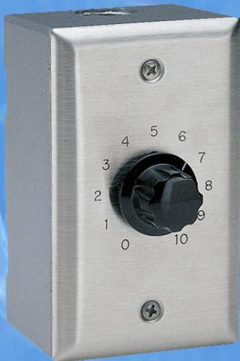
Clarity's 20-Watt Speaker Attenuator controls the volume of 25 or 70-volt speakers and horns. The attenuator consist of an auto-transformer and a 10-position switch that is mounted on a steel plate, has embossed numbers and fits a single gang electrical wall box.
