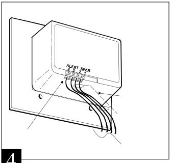
The Door Speaker back panel has two sets of terminals: one set is labeled SPKR and the other is labeled ALERT. The two ALERT terminals are labeled 3 and 4, and are connected to the doorbell input terminals of the Controller. The other two terminals (1 and 2) are labeled SPKR. The SPKR terminals connect to the output of the Controller and must use shielded twisted pair wire.
