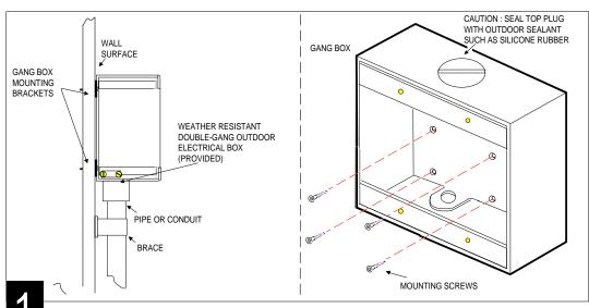
A The gang box mounting brackets (included) can be screwed to the gang box back plate so they protrude out the sides of the gang box. Using the appropriate screws (depending on the material the wall is made of), position the screws through the bracket holes and using a screwdriver secure the gang box to the wall surface. Once the gang box has been properly braced, install the speaker unit and face plate as shown in illustrations 4 and 5.
