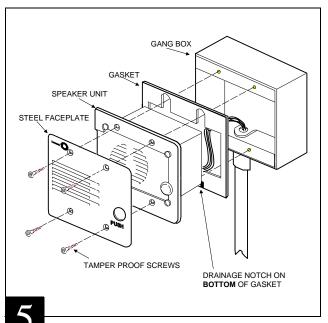
Use the allen wrench supplied to secure Door Speaker and faceplate to double-gang outlet box with the four tamper proof mounting screws. (included).
