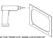
USING THE TEMPLATE, MARK LOCATION OF OPENING AND MOUNTING HOLES ON WALL. DRILL HOLES APPROPRIATE TO MOUNTING HARDWARE AND CUT OUT THE OPENING.
