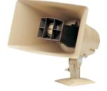
The V-1038 is a weather resistant, reentrant 30-watt amplified horn speaker, complete with 30-watt amplifier, volume control, horn housing, mounting base and I-beam clamp.
