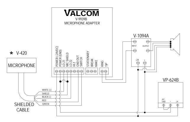
\*NOTE: V-400/450 and V-420 Microphones are wired differently. See correct diagram above.
