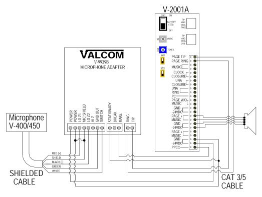
FIGURE 4 - OVERRIDE A SINGLE ZONE WITH A V-2001A
