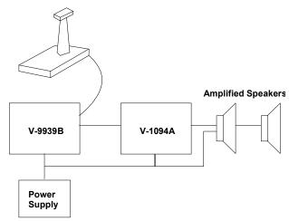
FIGURE 1 – BLOCK DIAGRAM OF A TYPICAL INSTALLATION
