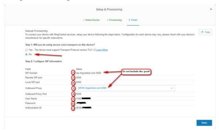
The key numbers indicate corresponding fields on the SIP tab of the V-9972 web interface.
