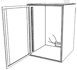
3) Remove the metal punch-outs so that cables can be installed. Thread the cables through the punch-out holes.
