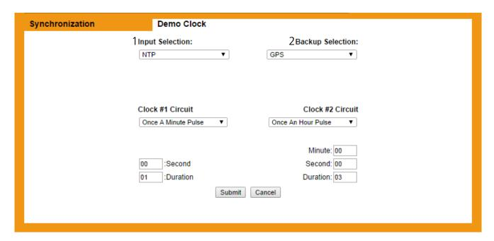
**1. Input Selection -** This drop-down list allows the user to select which service signal the master clock will depend upon for accurate time. The options include:
