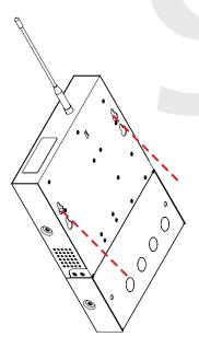
10) Pass the remaining two screws through the holes in the bottom compartment and into the wall anchors.
