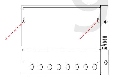
10) Pass the remaining two screws through the holes in the bottom compartment and into the wall anchors.
