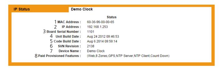
**NOTE:** Everything in this tab reflects settings entered earlier or hard-wired into the master clock. This page is view-only. None of these settings can be changed from this tab.
