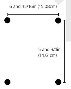
2) Use a drill to drill holes into the wall at the marked locations.
