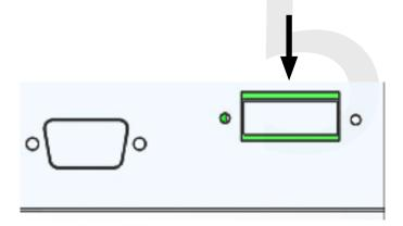
6) Use a screwdriver to reattach the master clock bottom panel.
