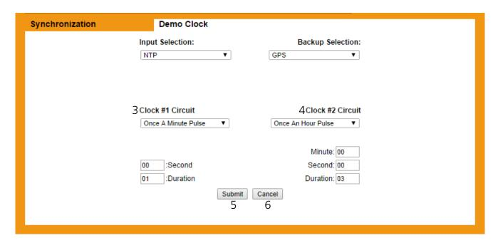
**3. Clock #1 Circuit -** This drop-down list allows the user to select the sync-wire output for master clock Sync-wire Circuit 1. The available output signals are:
