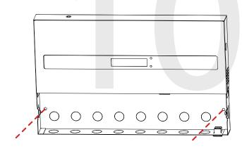
11) Use a screwdriver to reattach the master clock bottom panel. If your master clock has a wireless signal antenna, attach it to the port on top of the hardware case.
