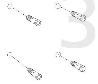
4) Insert the sheet metal screws into the top two wall anchors.
