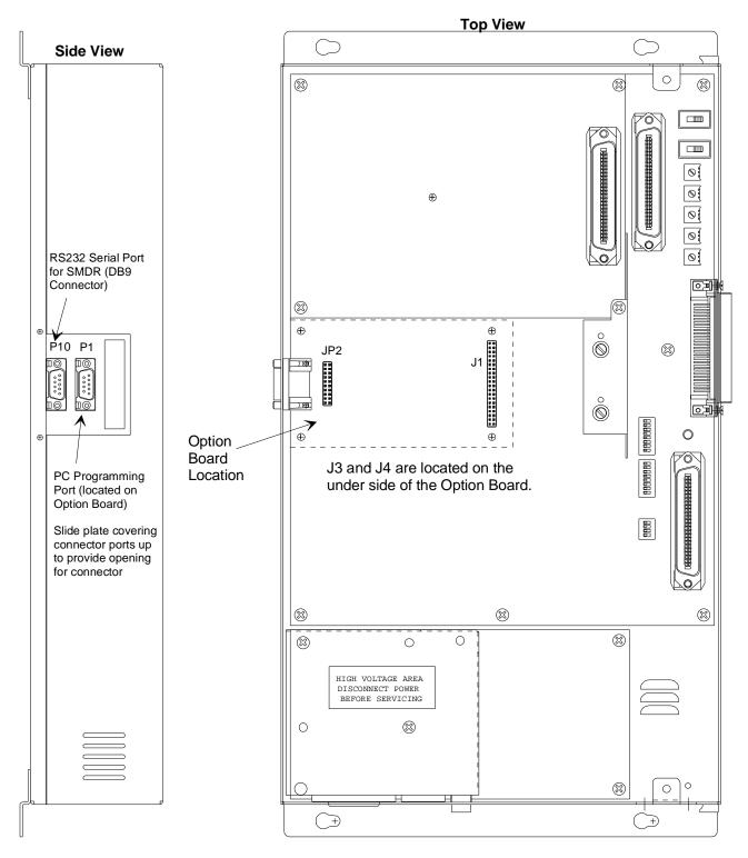
Align J3 on the Option Board directly over J1 on the Control Board Align J4 on the Option Board directly over JP2 on the Control Board Press Option Board firmly into place.
