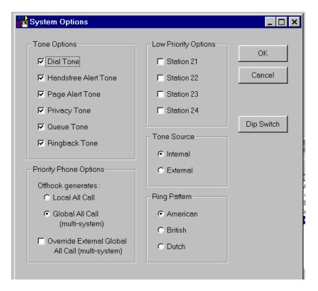
Dip switch equivalent of programmed options.
