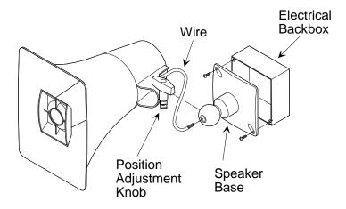
Figure 2 - Mounting to an Electrical Backbox
