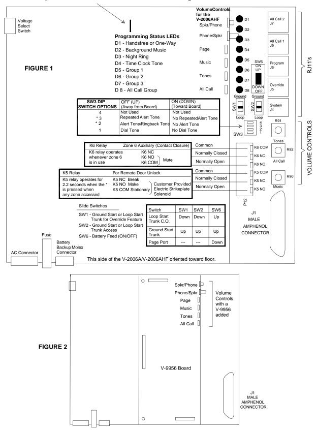
It is necessary to remove the JUMPER on the V-2006A board before connecting the V-9956 board to the V-2006A board.
