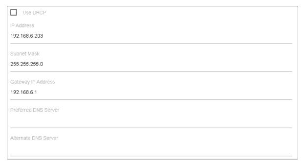
If the Use DHCP checkbox is <u>not</u> checked, the IP address information can be entered as static values. The web page will display fields for the IP Address, Subnet Mask and Gateway IP Address. The fields for DNS Server entries are optional, although other programming options for SIP may require the DNS entries to be entered.
