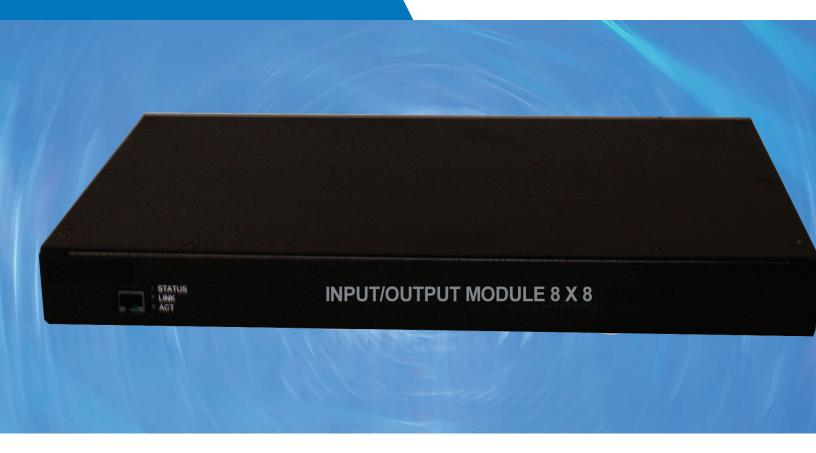
Valcom's InformaCast® IP Input/Output Module allows operation of eight (8) contact closures which are software programmable as either Form A or Form B. Eight (8) contact closure activated inputs provide for various programmable relay functions. The Input/ Output Module allows initiation of Application Serverevents over an IP based LAN/WAN.
