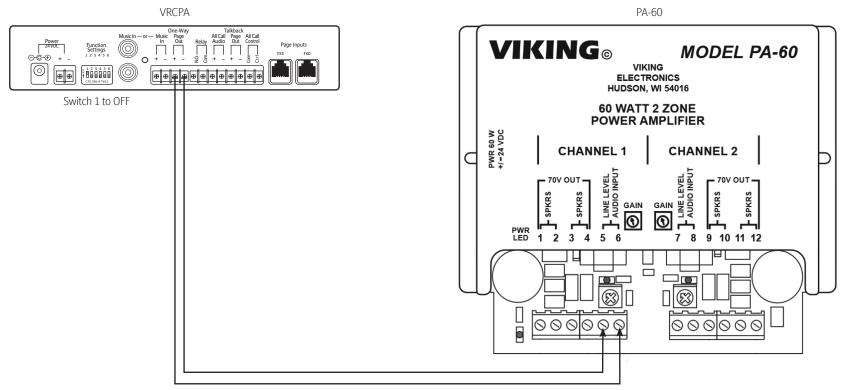
VRCPA audio may also be connected to Channel 2 or both Channels jumpered together.
