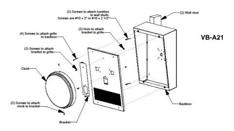
Figure 1. Assembly and Mounting
