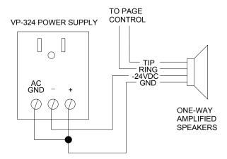
Connections to One-Way Amplified Speakers
