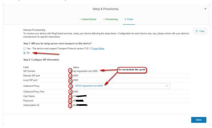
The key numbers indicate corresponding fields on the SIP tab of the VRCPA web interface.
